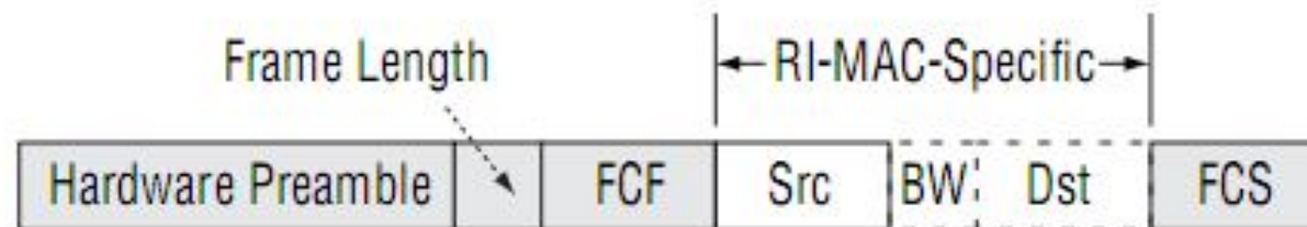
Figure 4: The format of an RI-MAC beacon frame for an IEEE 802.15.4 radio. Dashed rectangles indicate optional fields. The Frame Length, Frame Control Field (FCF), and Frame Check Sequence (FCS) are fields from IEEE 802.15.4 standard.
